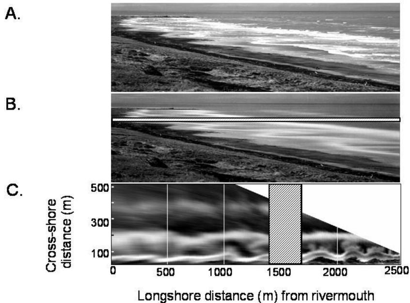
Figure 3 Examples of instantaneous (1/125<sup>th</sup> sec) photo (A), corresponding 4 min time-exposure photo (B), and rectified image with straightened coastline (C). Photo is the first in an 8 shot panorama. The 300 m wide study area is depicted by the shaded areas in B and C.
