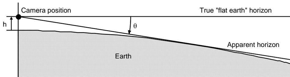
**Figure 3:** Error between true horizon and apparent horizon.
