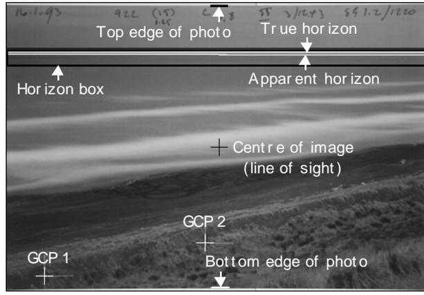
**Figure 5:** The input image with key features labelled.
