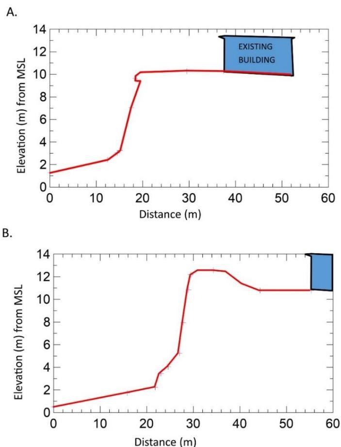
**Figure 3** Profiles for the eastern transect (A) composed primarily of volcanic ash, and the western transect (B) composed primarily of siltstone..
