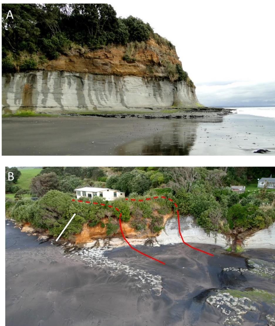
**Figure 2** Southern headland is depicted in photo A and the “site-embayment” fronting the Taylor property in photo B which also shows survey transects (red line) and the vegetated bank used to determine the stable slope angle for volcanic ash is marked by the white line
