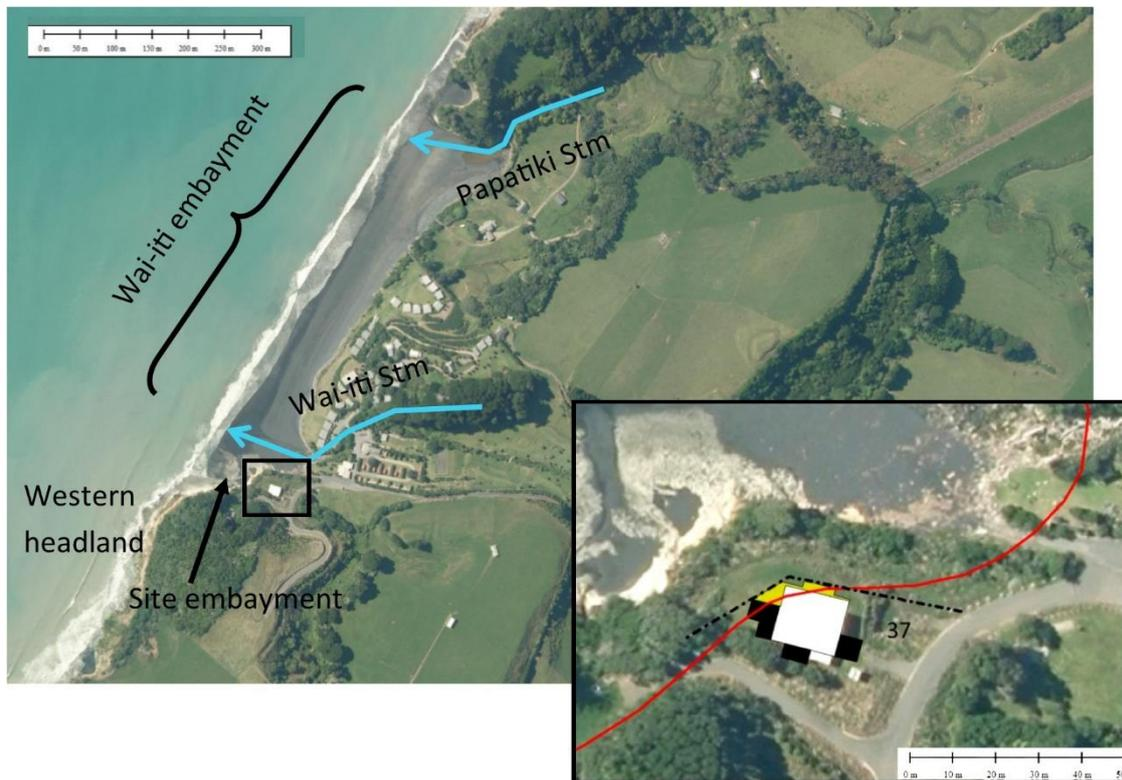
**Figure 1** Wai-iti Beach features and site (inserted) where the existing building is shown white, proposed modifications in black with proposed deck in yellow. The seaward property boundary is depicted by the black dash-dotted line, while the red line defines the current Area Susceptible to Coastal Erosion (ASCE) as defined in T&T (2018).
