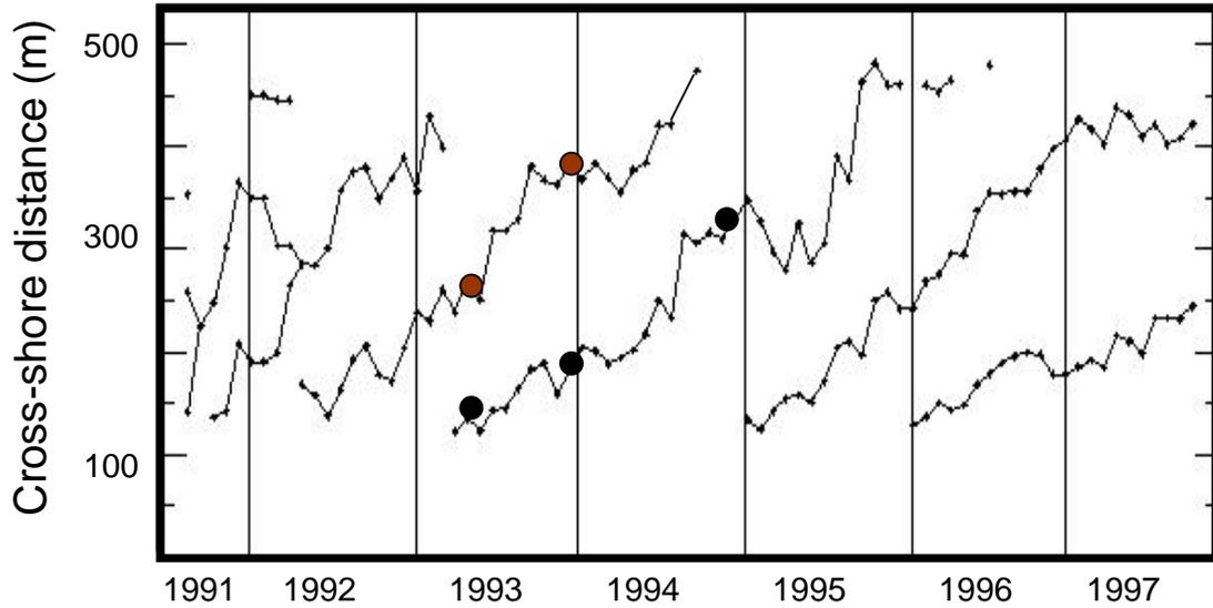
**Figure 5** Time-series of sub-tidal bar-crest locations for a 300 m wide transect centered 1550 m (from the rivermouth) during the period August 1991 to November 1997. The five dots locate the bar-crests depicted in the set of three time-lapse photos shown in Figure 4.
