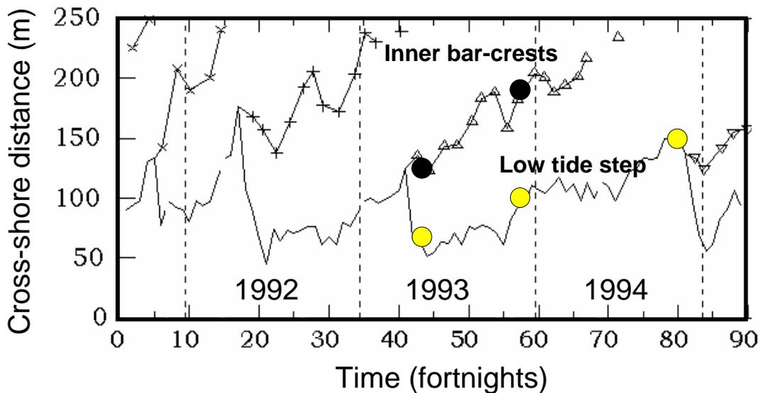
**Figure 6** Time-series of low tide step and inner bar-crests for 300 m wide transect centered 1550 m during the period August 1991 to March 1995. The five dots locate the step and bar-crests as depicted in the set of time-lapse photos shown in Figure 4.
