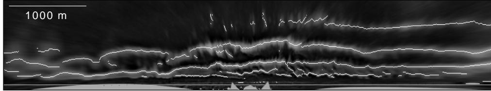
Figure 4: Detected sandbars and waterline (offshore distance scale x2)
