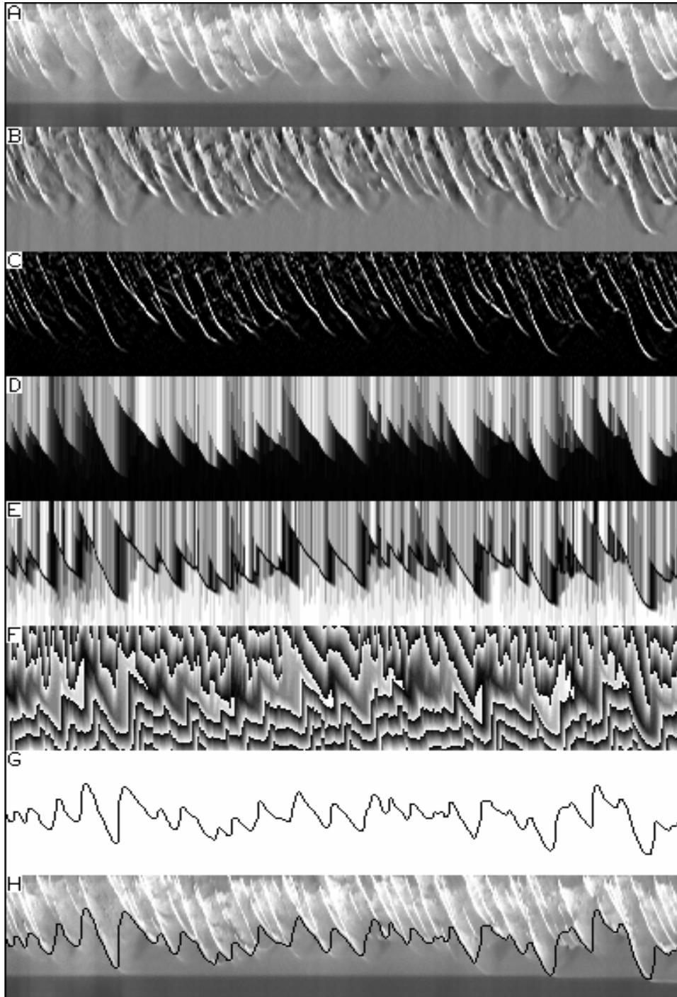
**Figure 4: Swash tracking sequence: A) cropped image; B) background removed; C) vertical edges; D) smeared upwards; E) tracking penalty function; F) path cost; G) least cost path, representing tracked swash; H) path overlaid on original**
