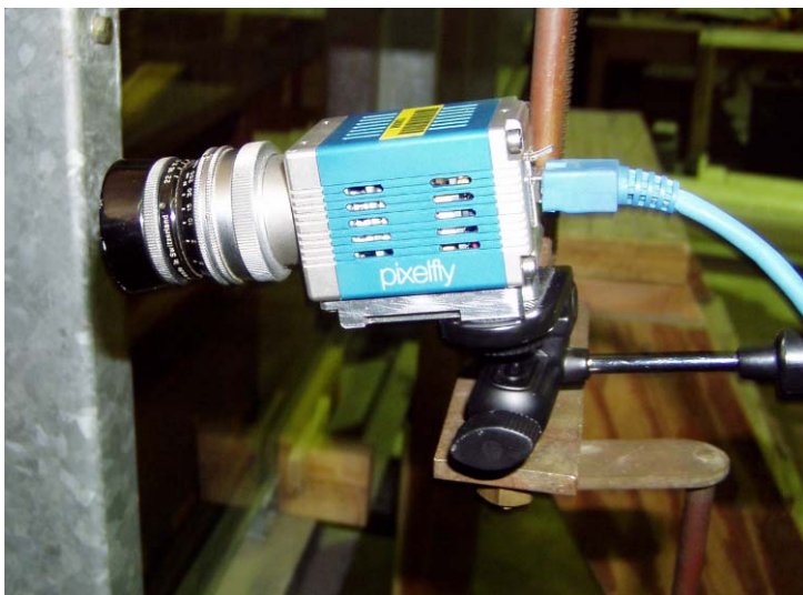
Figure 3-6 PixelFly 270XD CCD camera with Switar 25mm f/1.4 standard focal lens mounted to a flume-top trolley.
