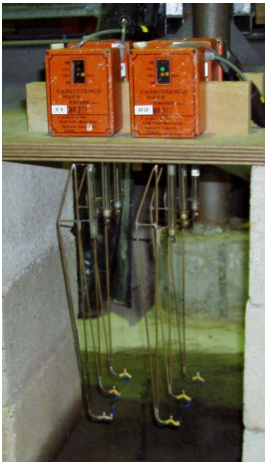
Figure 3-4 Capacitance-type wave probes used to capture water surface elevation.
