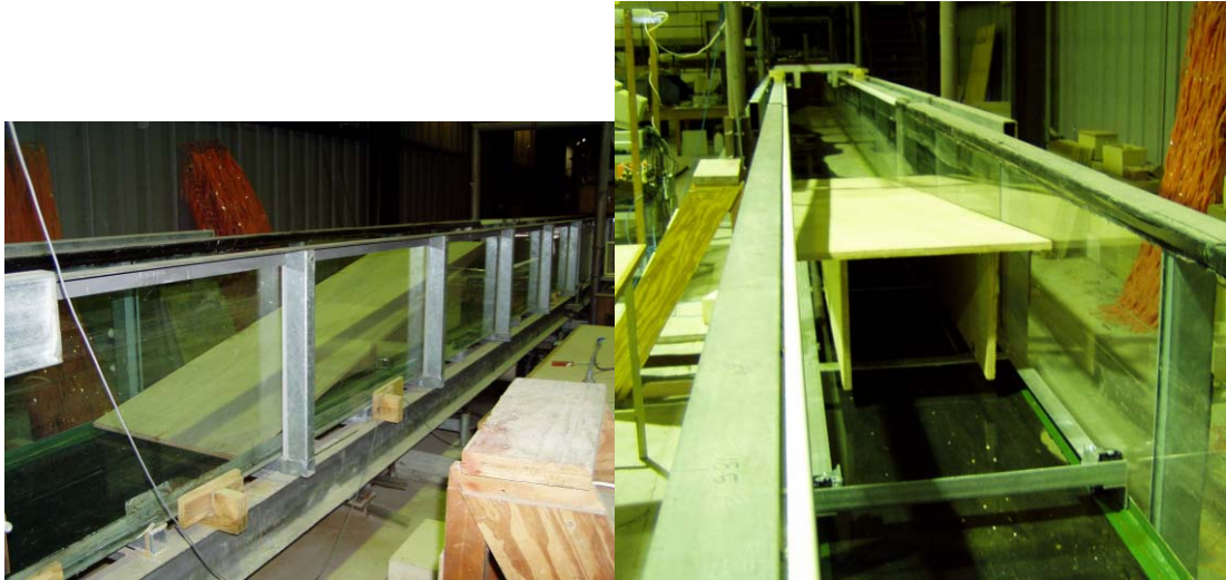
Figure 3-3 Sloping bed constructed on a moveable trolley within the flume.
