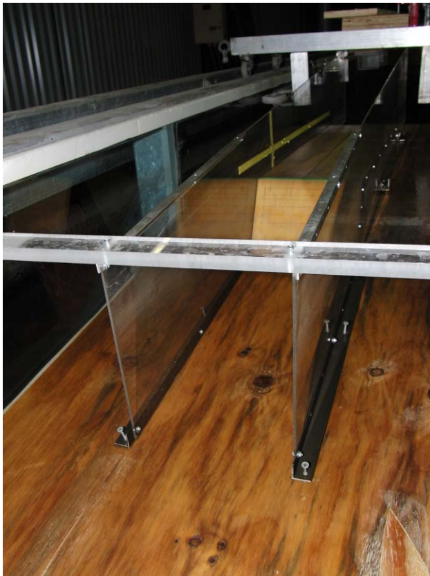
Figure 8-7 Photograph showing the model platform with perspex sidewalls sitting on the sloping bed. The instrumentation trolley can be seen in the background.
