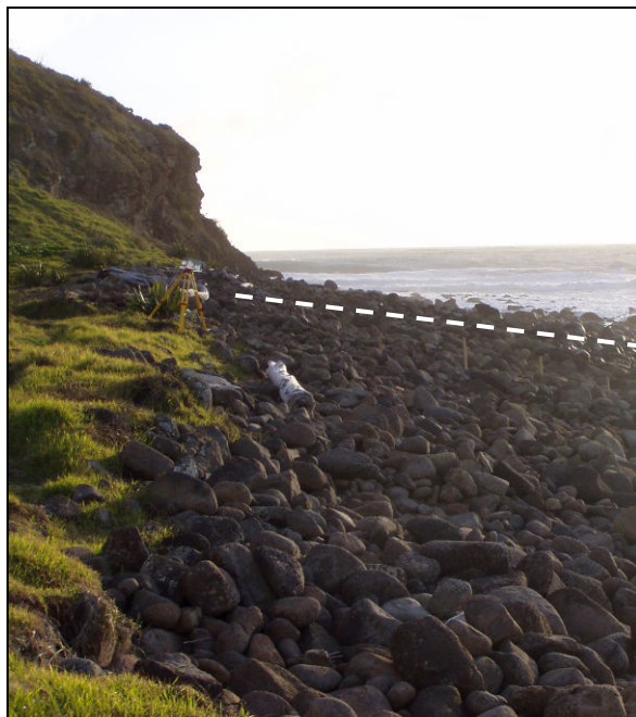
Figure 2 Video camera and run-up marker setup
