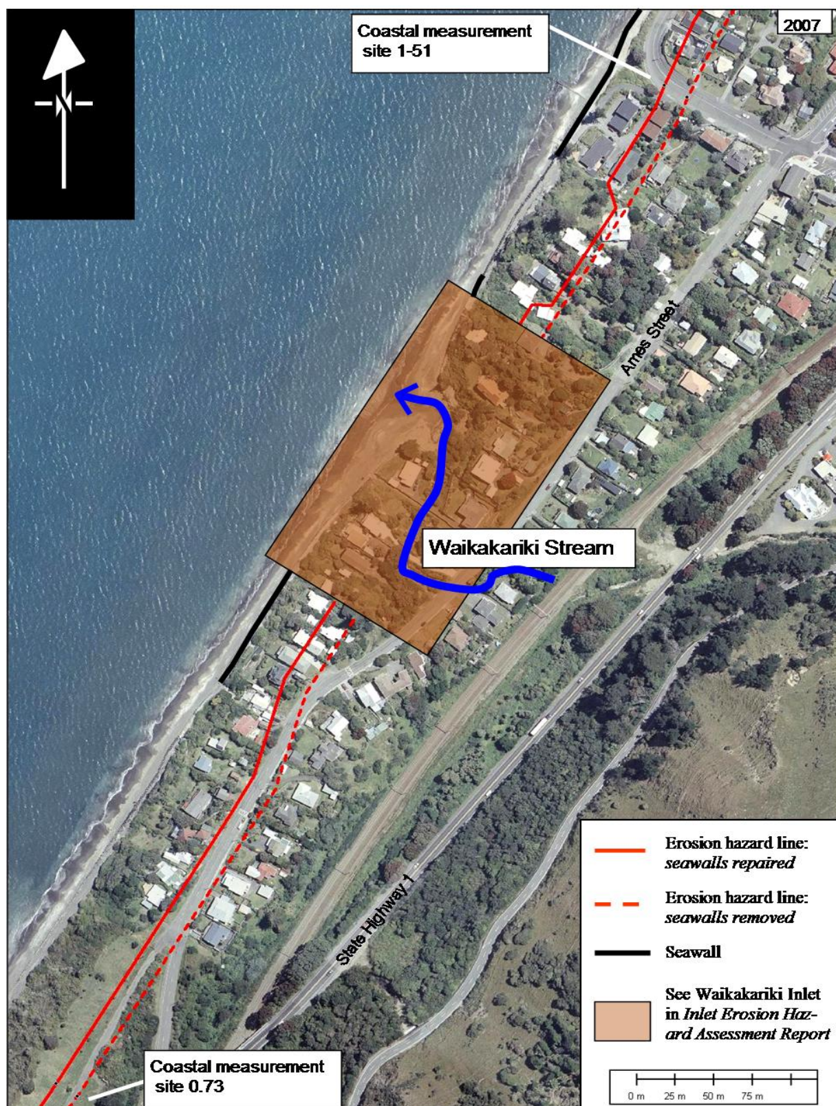
Fig 10 Example of erosion hazard lines for a partially seawalled stretch of coast at Paekakariki. The hazard lines relate to the seawalls repaired and seawalls removed scenarios (see text). The northernmost seawall was professionally designed and is maintained by the KCDC. The remaining partially seawalled coast contains a range of privately constructed and maintained structures. The depicted sections of seawall are approximate and used here to illustrate variation in the erosion hazard.
