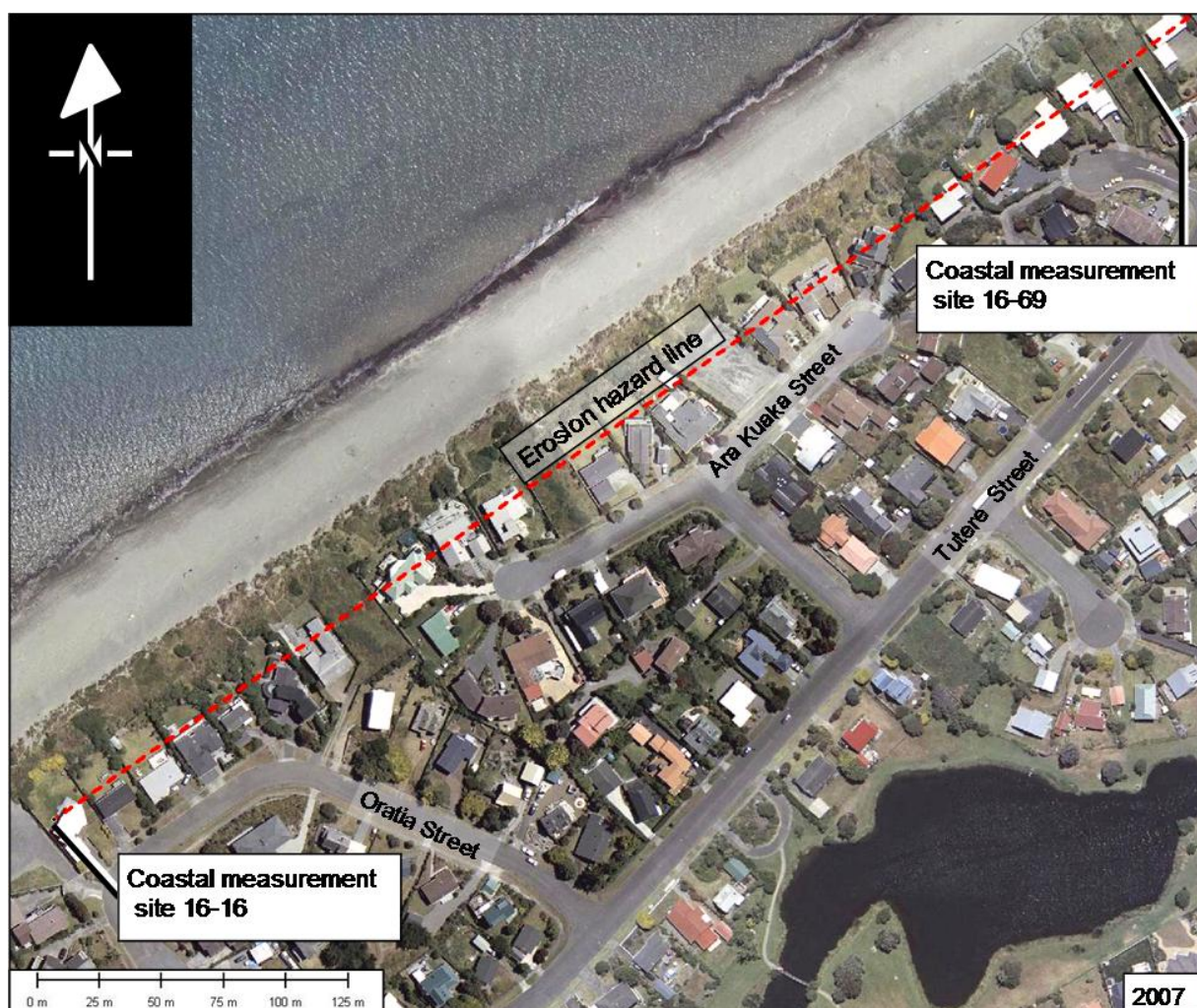
Fig 12 Example of an erosion hazard line along a natural stretch of open coast at Waikanae Beach. While sand conservation fencing has recently been constructed along part of the fore-dune, this does not affect the present erosion hazard assessment.
