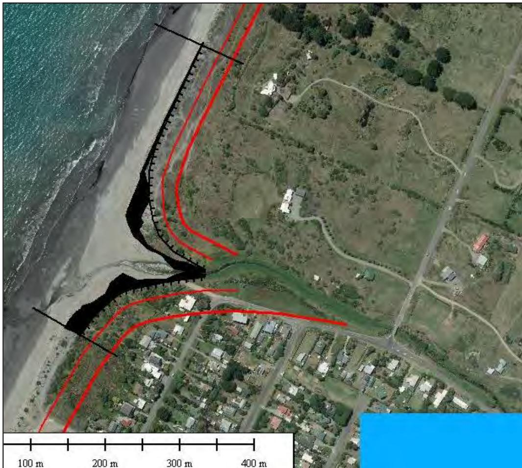
**Figure 1** Mangaone erosion assessment analysis for managed inlet 50 and 100 yr scenarios. The black areas depict the shoreline envelop for 1993 to 2013 samples out to the GWRC trigger lines (marked by black lines) used to initiate a mouth cut (realignment). The racked black lines define the inlet migration curves, while the thin and thick red lines define the 50 and 100 yr erosion hazard prediction lines respectively.
